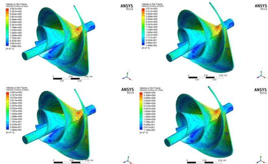
**Figure 14:** Velocity Contour(sth) at the velocity of 1.5m/s at 3rpm(top left), at 6rpm(top right), at 9rpm(bottom left) and 12rpm(bottom right)
