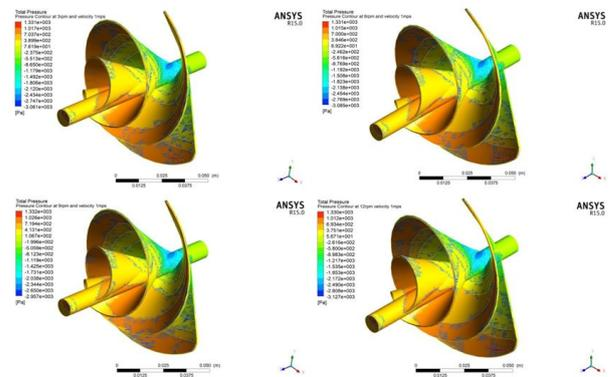
**Figure 10:** Pressure Contour at the velocity of 1m/s at 3rpm(top left), at 6rpm(top right), at 9rpm(bottom left) and 12rpm(bottom right)
