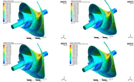
**Figure 13:** Velocity Contour(sth) at the velocity of 1m/s at 3rpm(top left), at 6rpm(top right), at 9rpm(bottom left) and 12rpm(bottom right)
