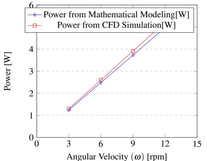
The power obtained from mathematical modeling and the CFD Simulation is plotted in graph 6 at the inlet velocity of 1.5m/s.
