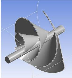
Figure 4: Isometric view of turbine blade in ANSYS
