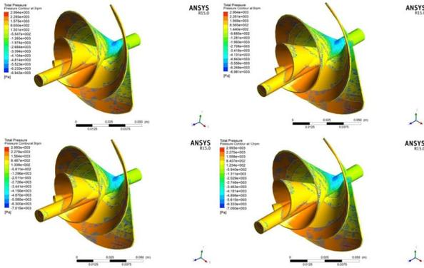
**Figure 11:** Pressure Contour at the velocity of 1.5m/s at 3rpm(top left), at 6rpm(top right), at 9rpm(bottom left) and 12rpm(bottom right)
