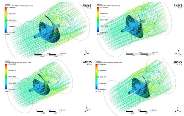
**Figure 9:** Streamline Flow at the velocity of 2m/s at 3rpm(top left), at 6rpm(top right), at 9rpm(bottom left) and 12rpm(bottom right)
