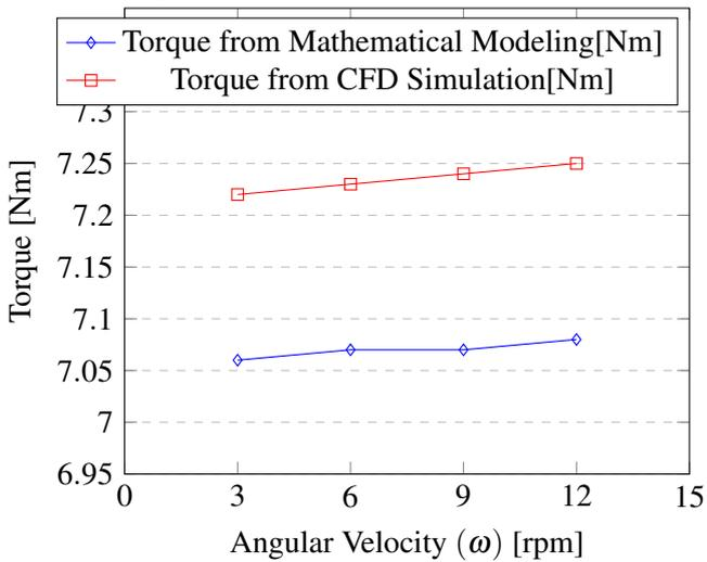
Graph 3 : Torque Obtained at velocity of 1.5m/s
