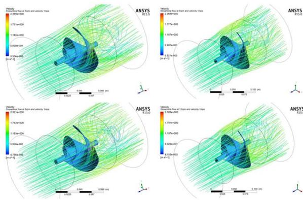
**Figure 7:** Streamline Flow at the velocity of 1m/s at 3rpm(top left), at 6rpm(top right), at 9rpm(bottom left) and 12rpm(bottom right)
