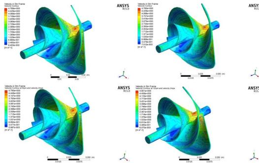
Figure 15: Velocity Contour(sth) at the velocity of 2m/s at 3rpm(top left), at 6rpm(top right), at 9rpm(bottom left) and 12rpm(bottom right)
