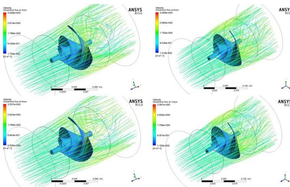
**Figure 8:** Streamline Flow at the velocity of 1.5m/s at 3rpm(top left), at 6rpm(top right), at 9rpm(bottom left) and 12rpm(bottom right)
