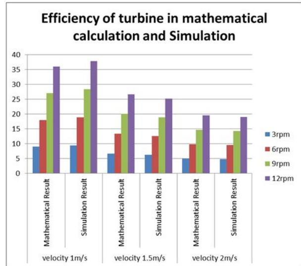
**Figure 16:** Efficiency of turbine in mathematical calculation and CFD Simulation
