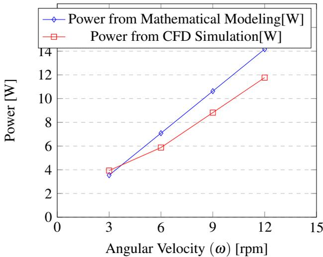
The power obtained from mathematical modeling and the CFD Simulation is plotted in graph 7 at the inlet velocity of 2m/s.
