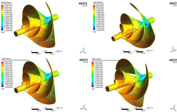
**Figure 12:** Pressure Contour at the velocity of 2m/s at 3rpm(top left), at 6rpm(top right), at 9rpm(bottom left) and 12rpm(bottom right)
