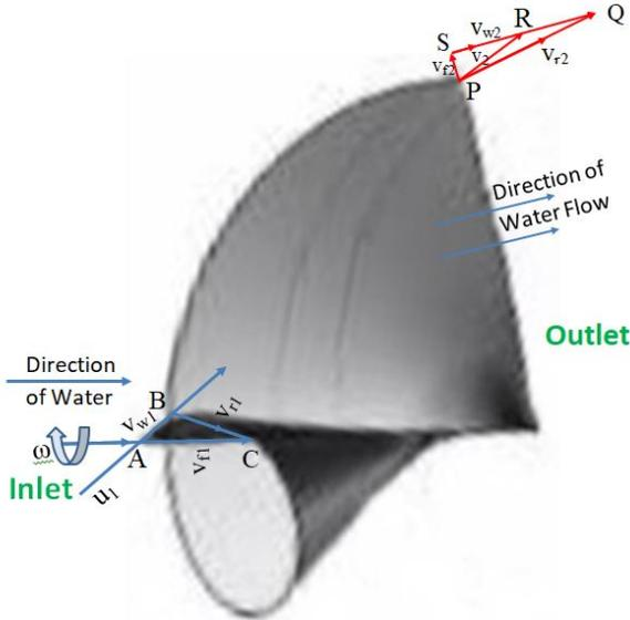
**Figure 3:** Velocity triangle at inlet and outlet
