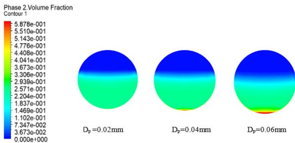
Figure 7: Outlet contours at different particle size
