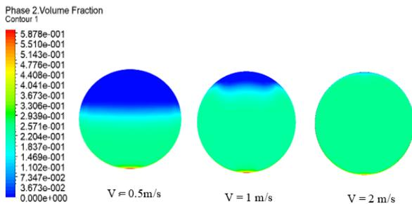
Figure 13: Contours at outlet for different velocity
