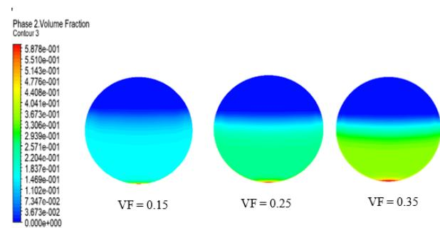
Figure 10: Outlet Contours at different initial volume fraction
