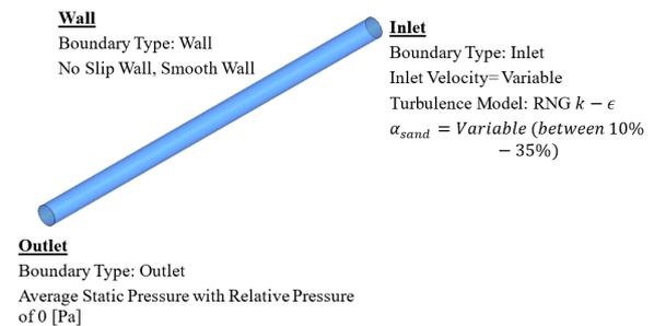
Figure 3: Boundary conditions for pipe
