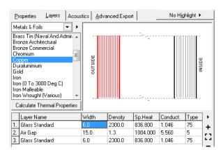
Figure 4: Double Glazing section detail
