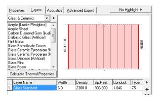
Figure 3: Single Glazing section detail
