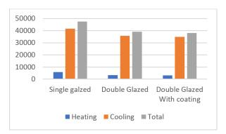
**Figure 7:** Energy performance of building according to glazed facade type
