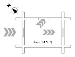
Figure 6: Provision of Cross Ventilation in Building
