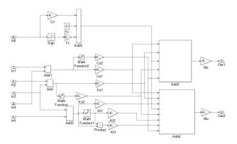
**Figure 6:** Subsystem for non-linear semi active suspension
