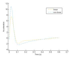
**Figure 10:** Acceleration curve for semi-active linear vs non-linear model
