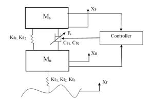
Figure 2: Semi active non-linear suspension system.
