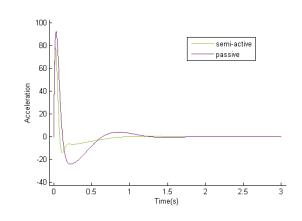
**Figure 8:** Acceleration curve for passive vs semi-active suspension
