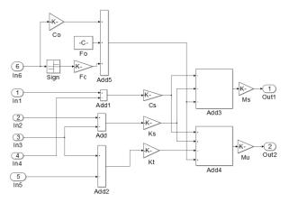
**Figure 5:** Subsystem for linear semi active suspension
