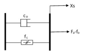
Figure 3: Bingham viscoplastic model of MR damper
