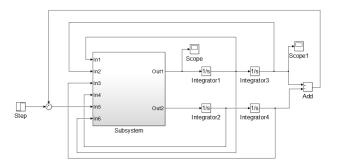
Figure 4: Semi active suspension SIMULINK model
