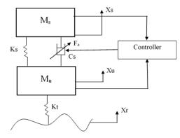
Figure 1: Semi active linear suspension system.
