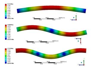
Figure 6: First three mode shapes from ANSYS
