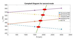
**Figure 10:** Variation of second mode natural frequency with rotational speed
