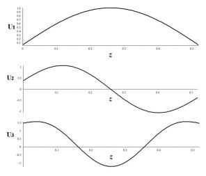
Figure 5: First three mode shapes
