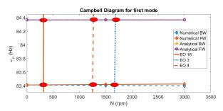
**Figure 9:** Variation of first mode natural frequency with rotational speed
