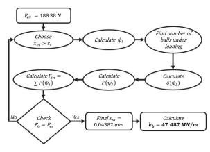
Figure 3: Stiffness of bearings
