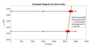
**Figure 11:** Variation of third mode natural frequency with rotational speed
