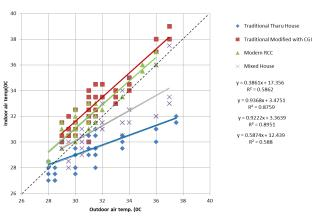
**Figure 11:** Regression analysis of indoor and outdoor air temperature of four different houses in summer
