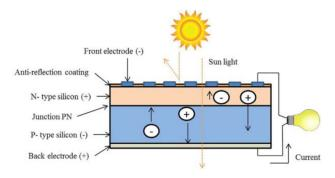
Figure 2: Photovoltaic Cell
