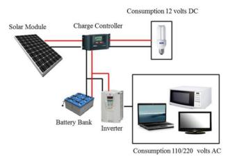
**Figure 3:** Typical System of Photovoltaic Solar Energy
