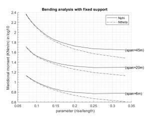
**Figure 11:** membrane stresses for fixed span spherical shells with different rise/span ratio for fixed support
