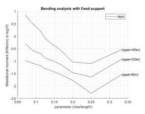
Figure 12: Moment stresses for fixed span spherical shells with different rise/span ratio for pinned support
