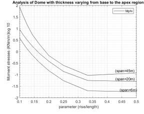
**Figure 14:** moment stresses for spherical shells with different rise/span ratio for edge beam with gradually varying thickness
