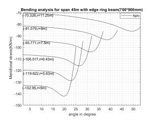
**Figure 5:** meridional stresses for the spherical shells with span 45 m supported on edge ring beam
