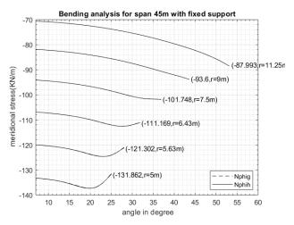
**Figure 1:** meridional Stresses for clamped support spherical shells with fixed span 45m and different rises
