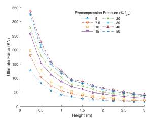
**Figure 5:** Ultimate force versus height for different precompression ratios
