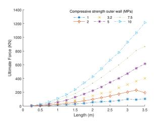
**Figure 6:** Ultimate force versus length for different compressive strength
