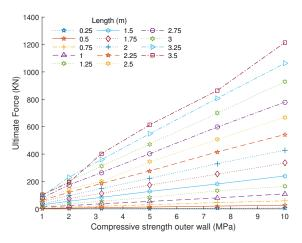
**Figure 8:** Ultimate force versus compressive strength for different lengths
