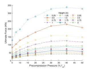
**Figure 9:** Ultimate force versus precompression ratio for different heights
