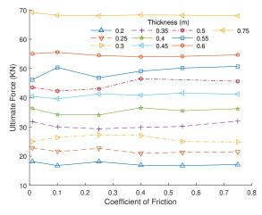
**Figure 10:** Ultimate force versus coefficient of friction for different thicknesses
