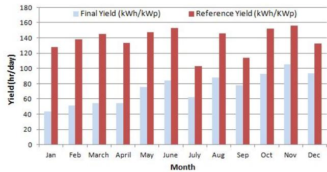
**Figure 7:** Measured monthly reference and final yield for the year 2016
