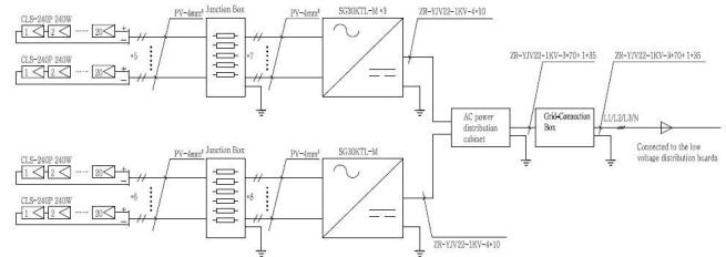
**Figure 5:** Single line diagram
