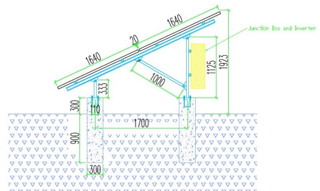
Figure 2: Mounting structure of PV panels
