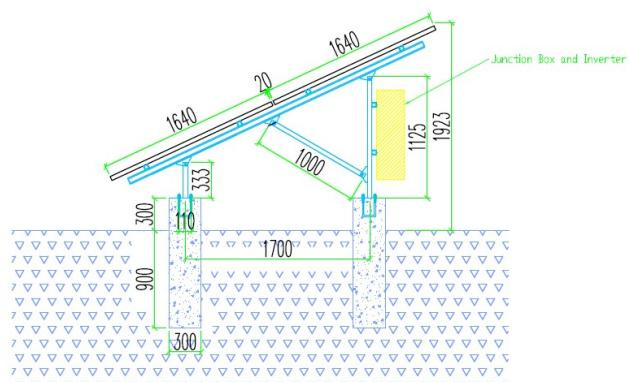
**Figure 2:** Mounting structure of PV panels
