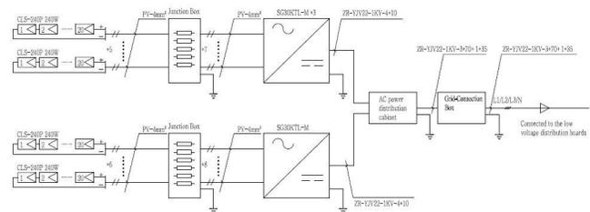
Figure 5: Single line diagram
