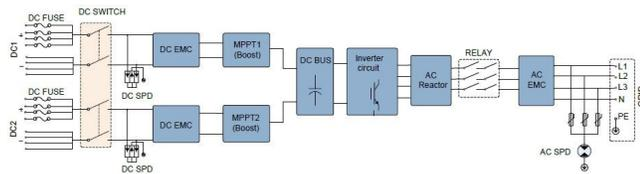
**Figure 6:** Circuit diagram of SG30KTL-M PV grid connected inverter
