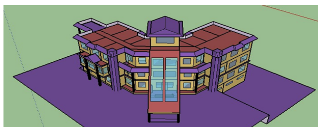
Figure 3: Energy model of Study Project-CES-Zero Energy Building
