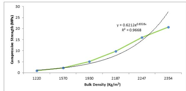
**Figure 7:** Relation of Bulk Density with compressive strength of concrete
