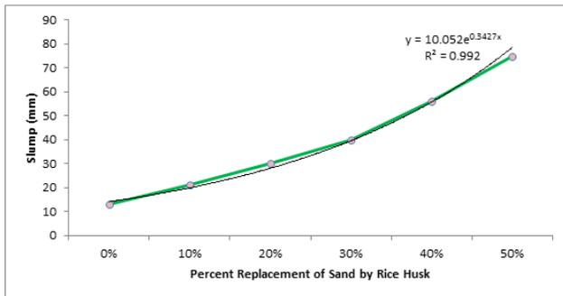
**Figure 1:** Variation of Slump of Fresh Concrete containing different percentage of Rice Husks
