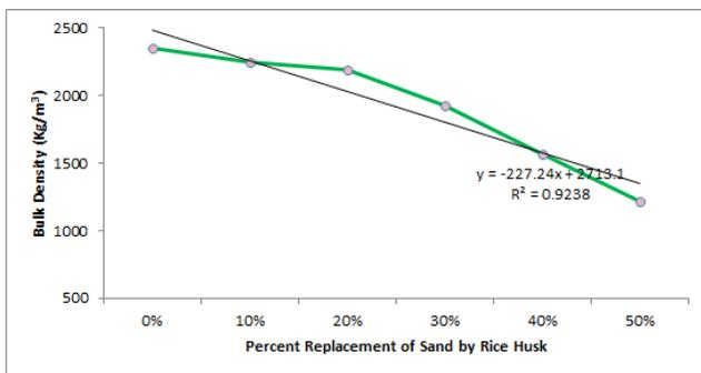
**Figure 2:** Variation of Bulk Density of Concrete containing different percentage of Rice Husks
