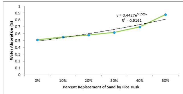
**Figure 3:** Variation of Water Absorption of Concrete containing different percentage of Rice Husks
