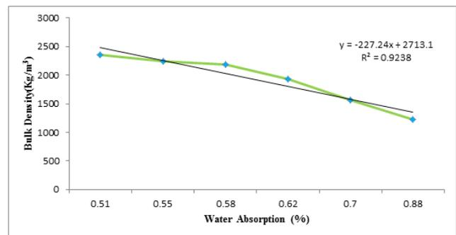
**Figure 8:** Relation of Water Absorption with Bulk Density of concrete
