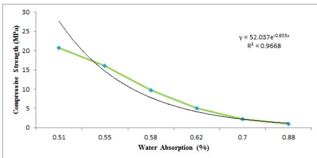
**Figure 6:** Relation of Water Absorption with Compressive Strength of concrete
