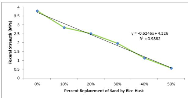
**Figure 5:** Variation of Flexural Strength of Concrete containing different percentage of Rice Husks
