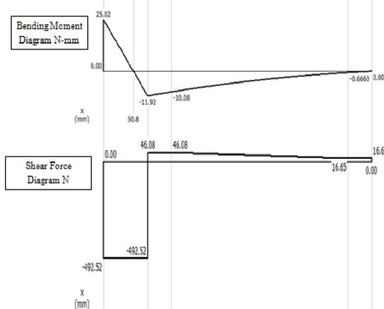
Reaction calculation of main shaft in x-z plane
