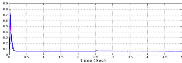
Figure 13: Total Harmonic Distortion of inverter current
