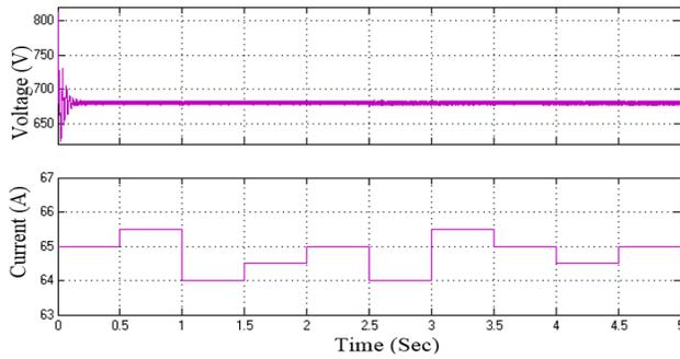
**Figure 7: DC Link voltage and inverter input current waveform**
