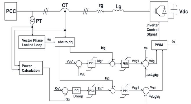
**Figure 5: Overall control structure of inverter**
