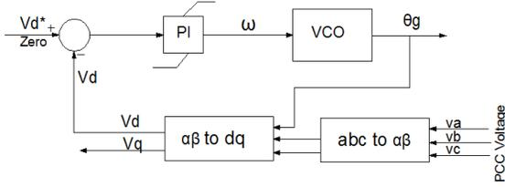
**Figure 4: Structure of the PLL system implemented in dq reference frame**
