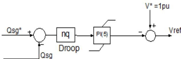
Figure 6: Reactive Power Drop of SG
