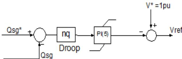
Figure 6: Reactive Power Drop of SG
