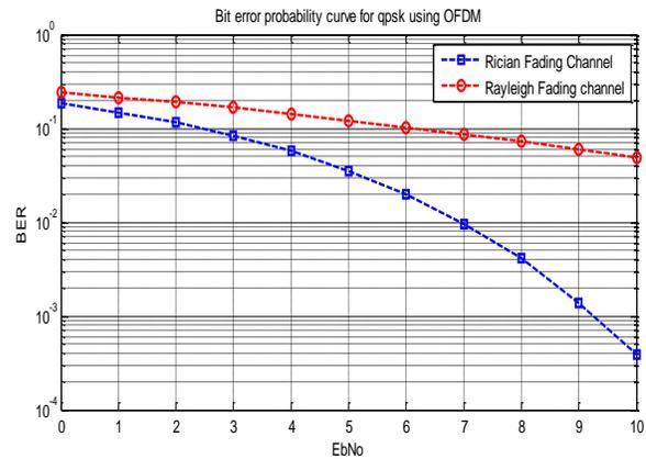
Figure 8.2: Simulation Plot using QPSK Modulation technique under different channel for Doppler shift
