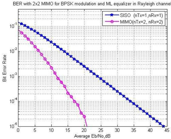
Figure 8.4:  $E_b/N_0$  Plot with ML estimation (2\*2)
