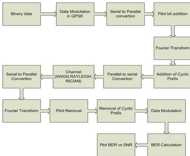
Figure 8.1: Block Diagram of simulation process
