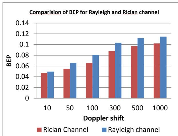
Figure 8.3 Chart for comparison of BEP for different channel due to different Doppler shift
