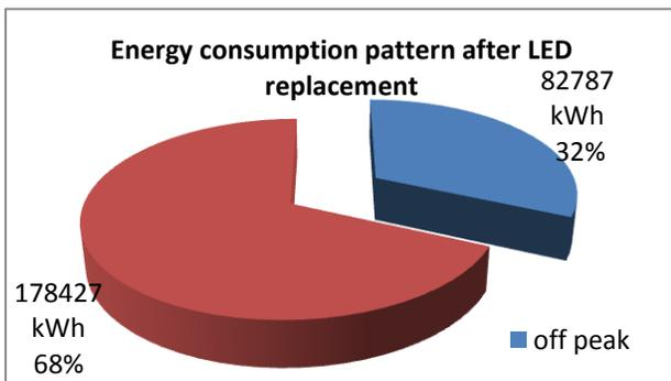
Figure 16: Energy consumption pattern for lighting in peak and off peak period after replacement of all bulbs by the LEDs
