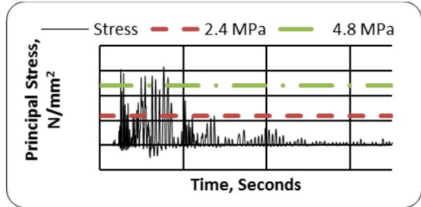
**Figure 8: Time history of major principal stress at the heel of the dam for Imperial Valley-06 (Recording station: El Centro Array#6) Earthquake (FN + V)**
