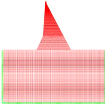
Figure 3: Dam-foundation model in SAP2000
