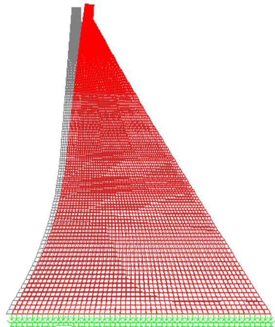
Figure 13: Dam finite-element model with gap-friction elements
