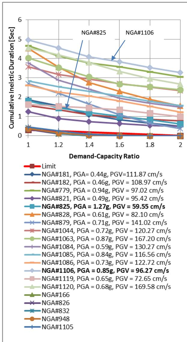
Figure 10: Comparison of cumulative duration of stress cycle with acceptance stresses at the heel of the dam
