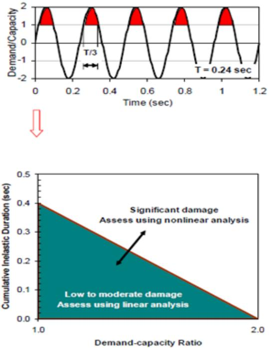
Figure 5: Basis for upper limit demand-capacity ratio and cumulative inelastic duration
