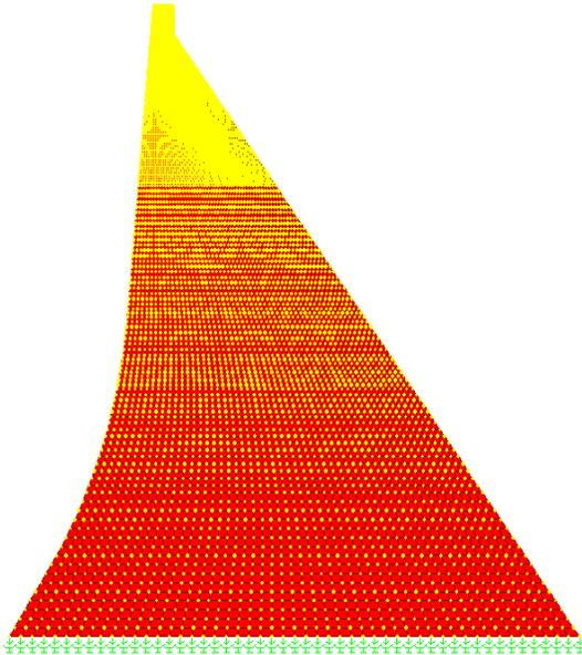
Figure 11: Dam finite element model with gap-friction elements
