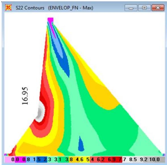
**Figure 6: Envelope of maximum vertical stresses (N/mm<sup>2</sup>) for proposed section.**
