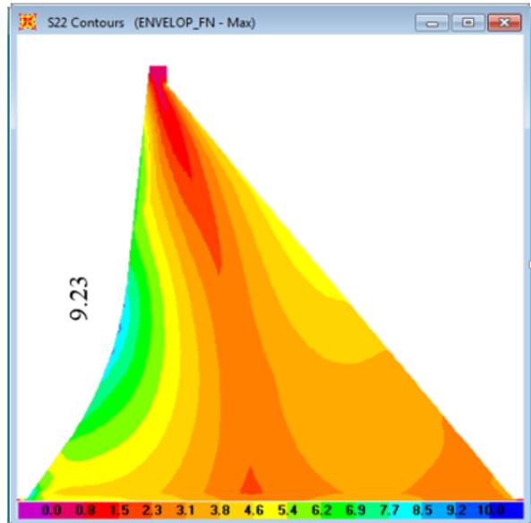
**Figure 7: Envelope of maximum vertical stresses (N/mm<sup>2</sup>) for proposed section**
