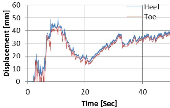
**Figure 14: Time history of sliding displacements of nodal points (heel and toe) at the base of dam (NGA#1120)**
