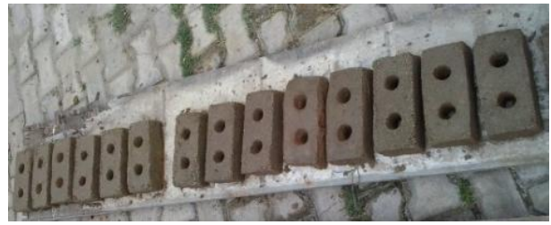
Figure 7: Fabrication of brick with two circular holes
