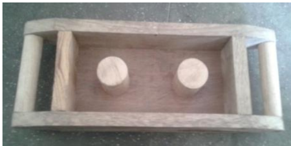
Figure 6: Mold selection for brick with air gap
