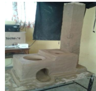
Figure 9: Fabricated two pot raised cook stove with modified brick
