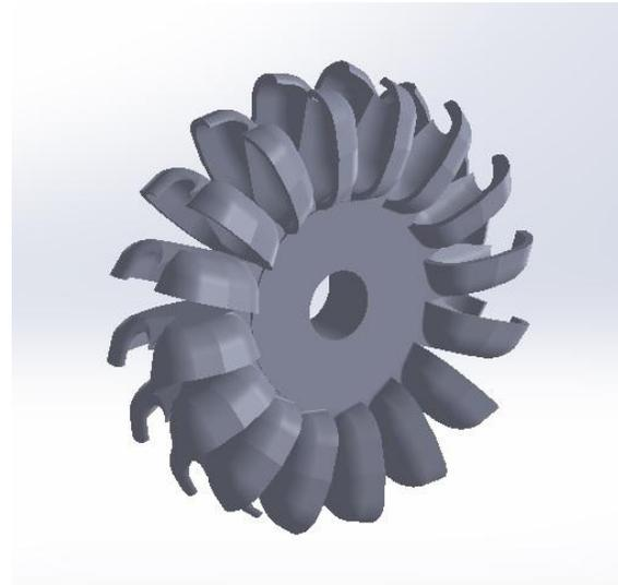
Figure 2: Pelton Turbine Model
