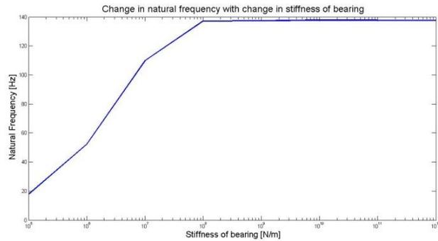
Figure 8: Simulation result of variation of natural frequency with change in stiffness of bearing
