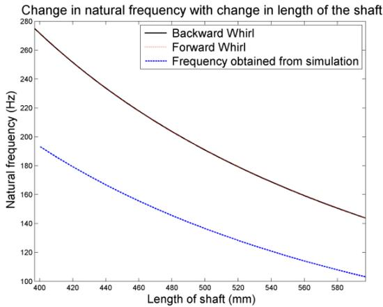
Figure 6: Variation of natural frequency with change in length of shaft
