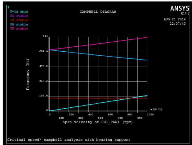
Figure 5: Campbell Diagram with consideration of bearing stiffness
