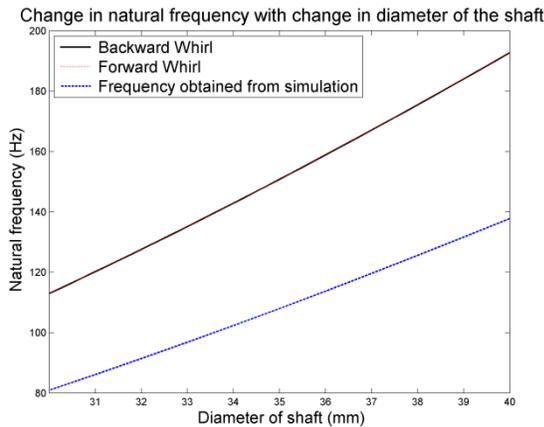
Figure 7: Variation of natural frequency with change in diameter of shaft
