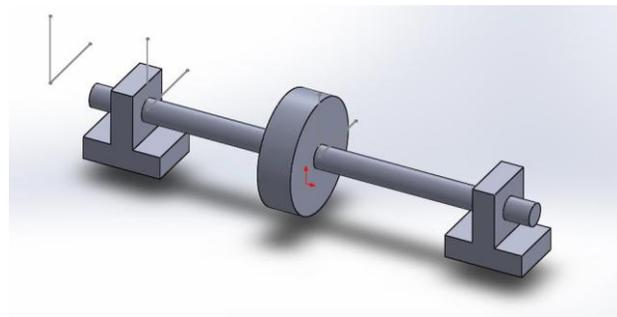
Figure 1: Simple Rotor Disk System
