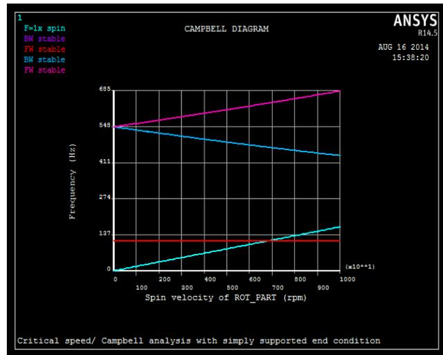
Figure 4: Campbell Diagram with rigid support
