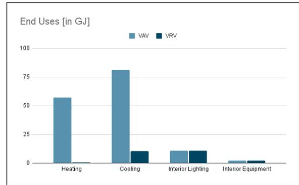
Figure 4: End Uses Comparison of VAV and VRV
