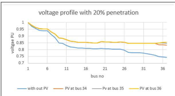
**Figure 10:** voltage profile with 20% penetration without kVAR supply
