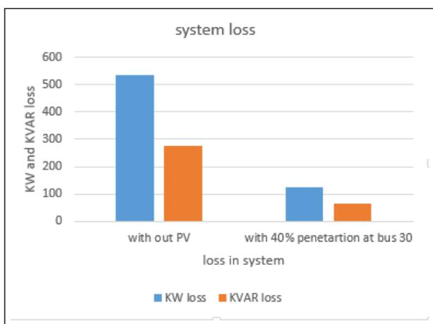
**Figure 13:** system loss at 40% penetration
