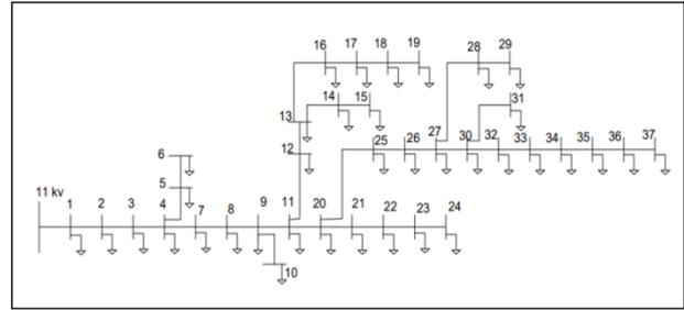
**Figure 1:** Single line diagram of 37 bus Rajgadh feeder
