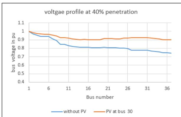
**Figure 12:** voltage profile at 40% penetration
