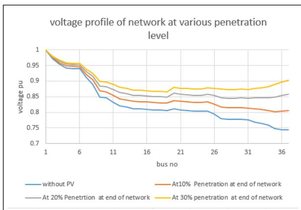
**Figure 5:** voltage profile of network at different penetration level
