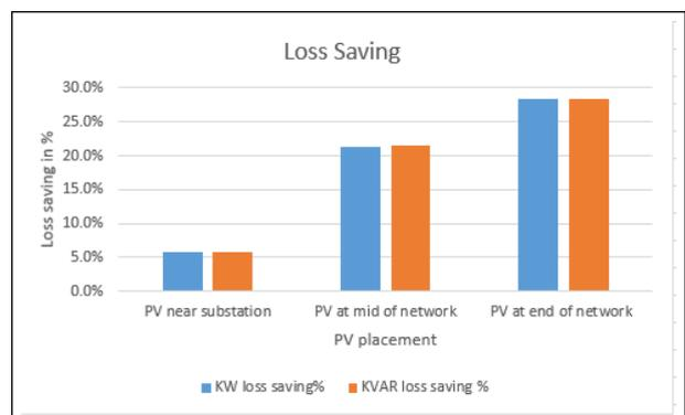
Figure 4: loss saving with PV penetration at different location
