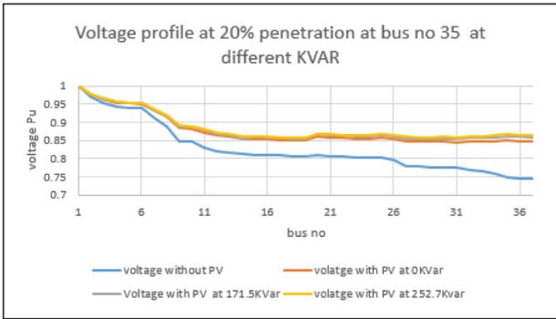
**Figure 8:** Voltage profile at different reactive power
