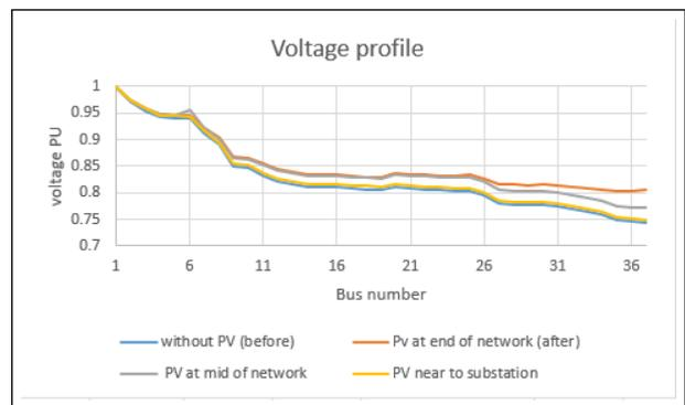
Figure 3: voltage profile of Network at 10% penetration at three different location
