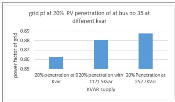
**Figure 7:** power factor of supply grid
