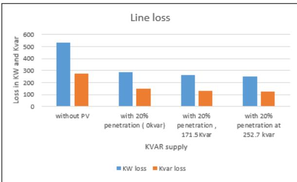
**Figure 9:** line loss at different reactive power
