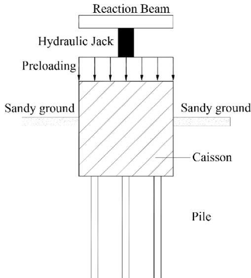
**Figure 3:** Experimental setup for vertical loading test [10]
