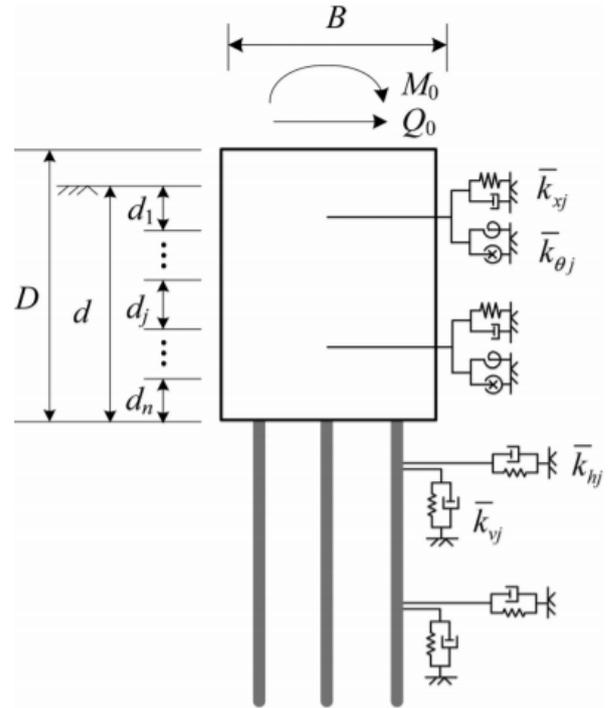
**Figure 6:** A sample numerical model of the composite foundation based on the BNWF [14]
