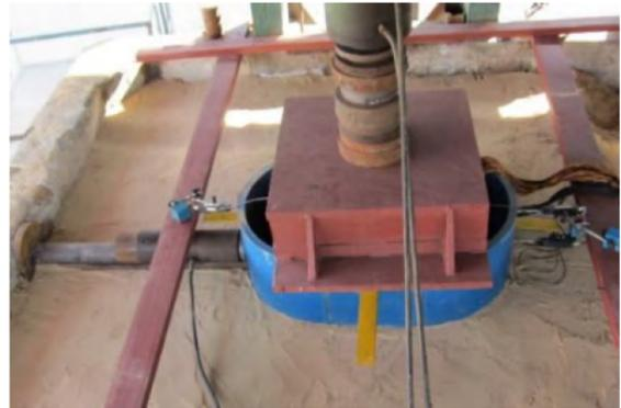
**Figure 4:** Overall layout of horizontal load test [11]
