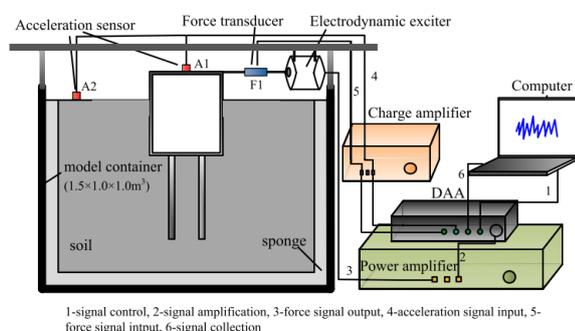
**Figure 9:** The excitation test schematic diagram performed by Tu et al. [23]
