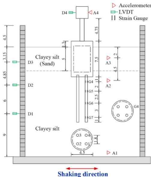
**Figure 8:** Schematic front view of the CWPF model with 2 × 2 piles and the instruments in the centrifuge tests carried out by Zhang et al. [16] (prototype scale, dimensions in m)
