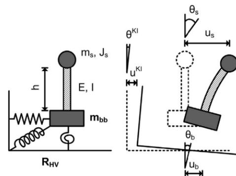
**Figure 7:** Simplified model for the interaction of CWPFs with structures, as well as the lateral deformation of this model [15]
