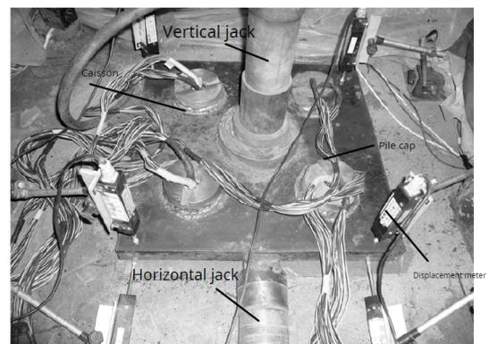
**Figure 5:** Schematic diagram of combined horizontal and vertical loading setup [12]
