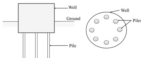
**Figure 2:** A sample layout of composite well-pile foundation (CWPF) system
