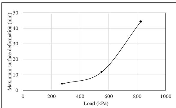
**Figure 8:** Surface deformation for unreinforced pavement at different loading condition
