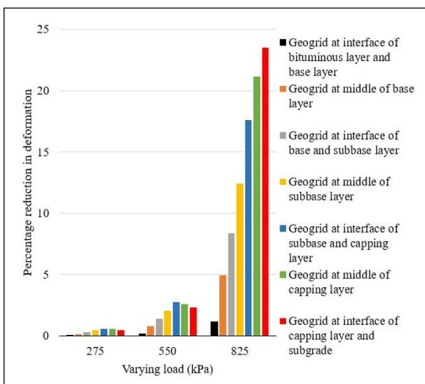
**Figure 9:** Percentage reduction in surface deformation due to inclusion of geogrid at varying wheel load
