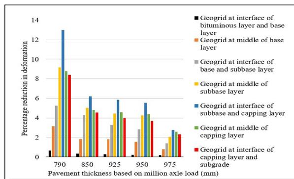
**Figure 6:** Percentage reduction in surface deformation in geogrid reinforced pavement compared with unreinforced pavement
