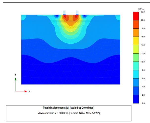
**Figure 3:** Surface deformation in the unreinforced pavement of thickness 790mm
