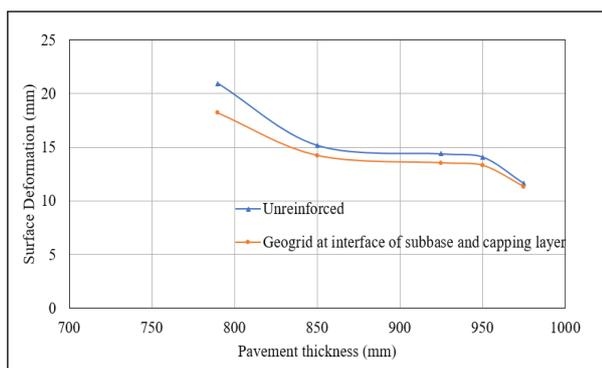
**Figure 5:** Surface deformation in the pavement for different pavement thickness
