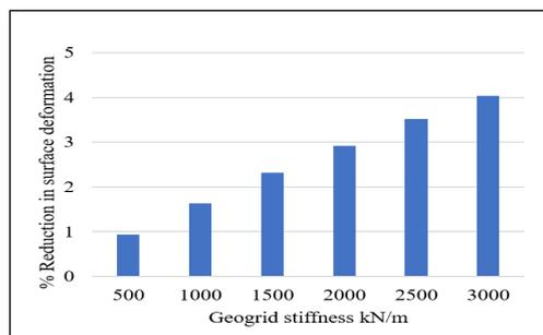
**Figure 7:** Percentage reduction in surface deformation at varying geogrid stiffness
