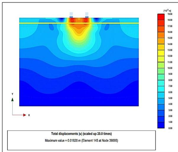
**Figure 4:** Surface deformation in geogrid reinforced at the interface of subbase and capping layer with pavement thickness of 790mm
