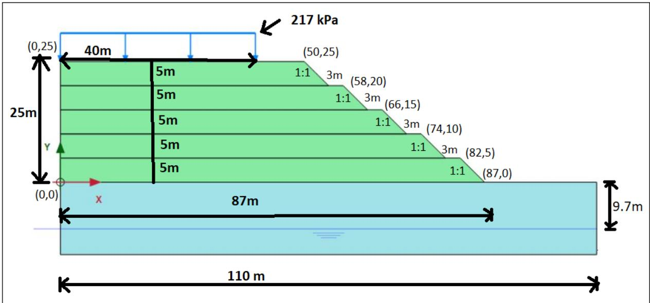
Figure 1: Geometry of the Model (without Geogrid)
