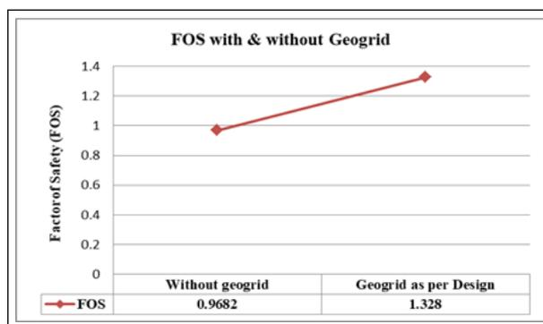
**Figure 3:** Variation of FOS of Embankment with and without Geogrid
