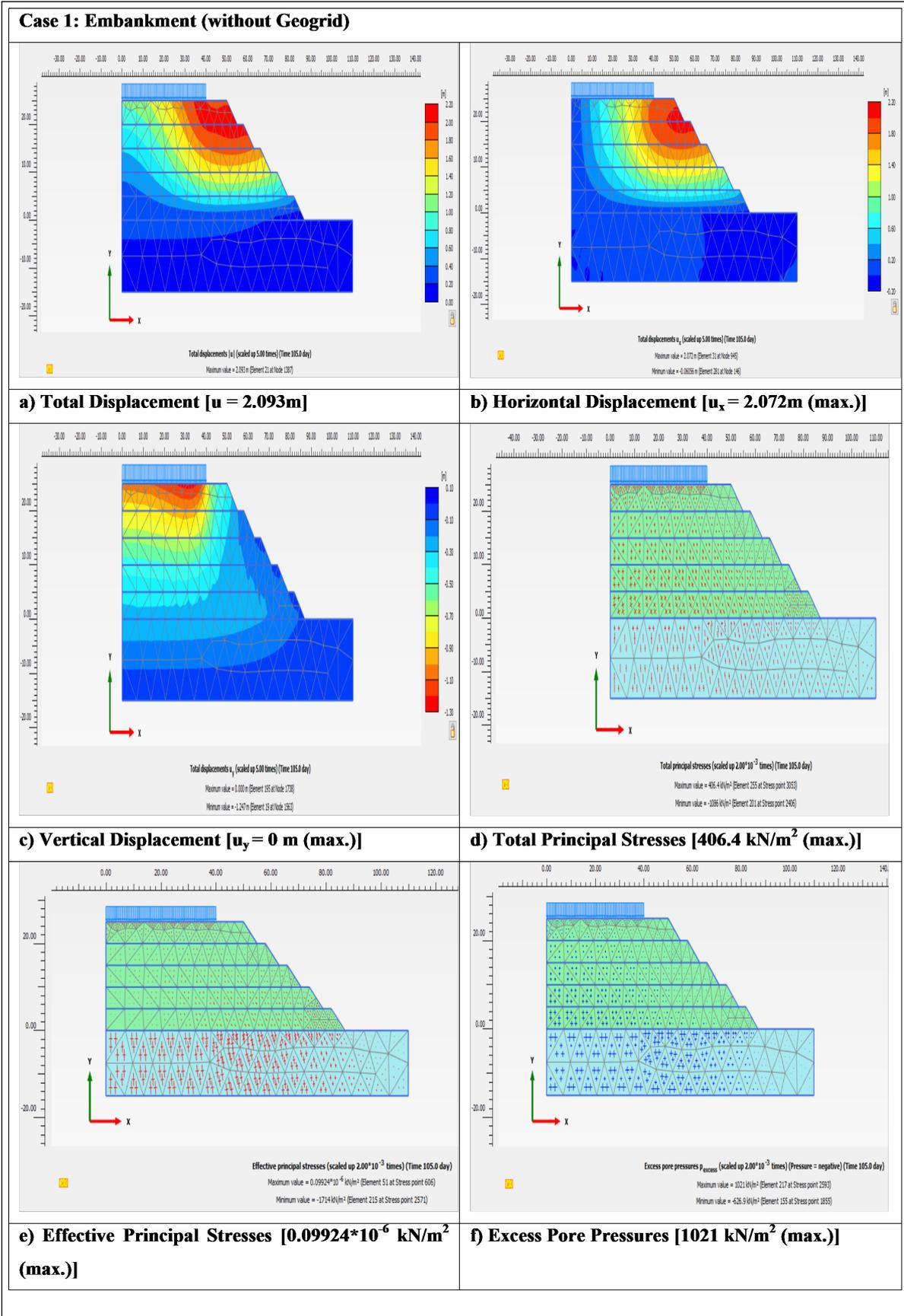
Figure 5: Deformations and Stresses (Embankment without Geogrid)
