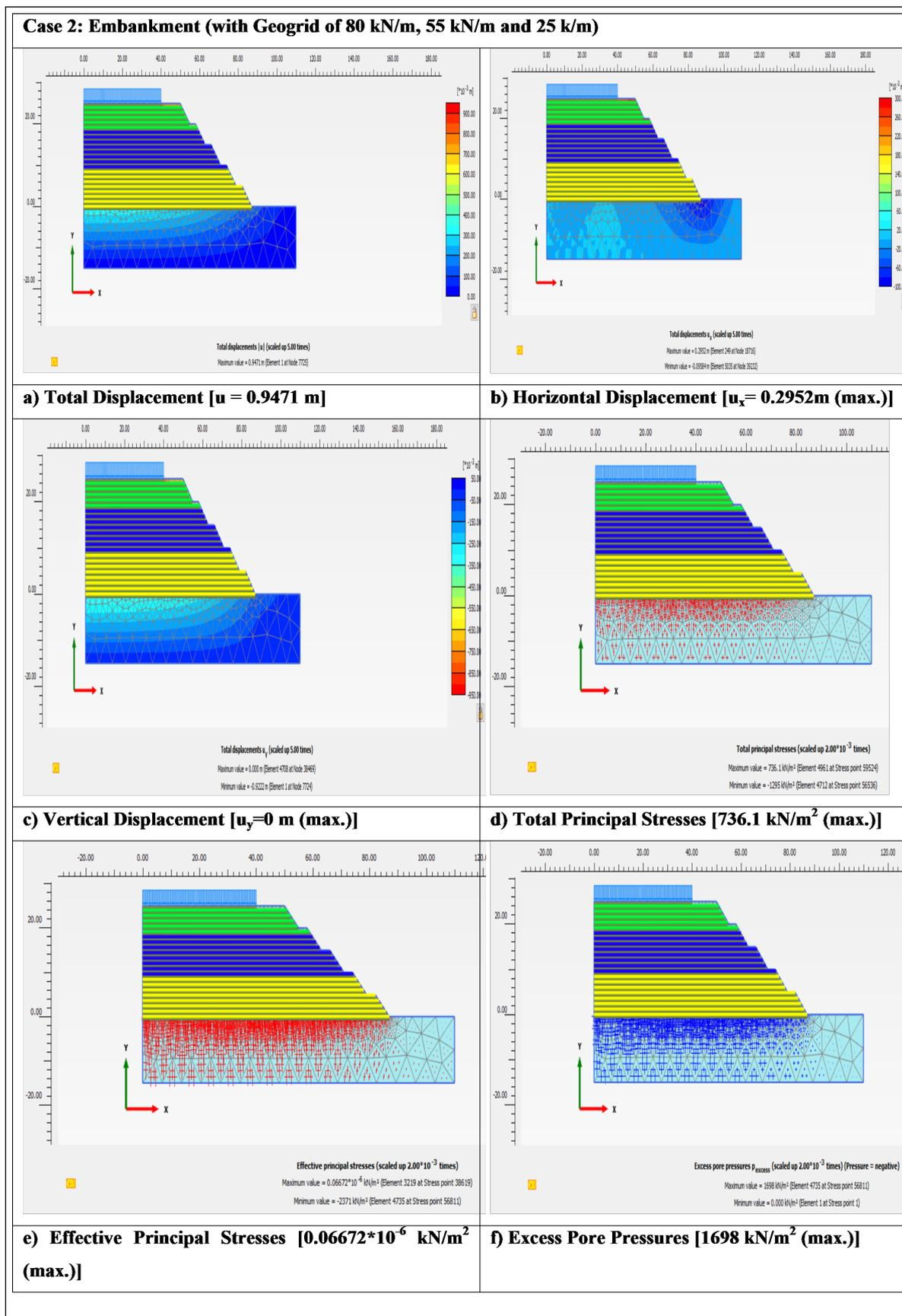
Figure 6: Deformations and Stresses (Embankment with Geogrid)
