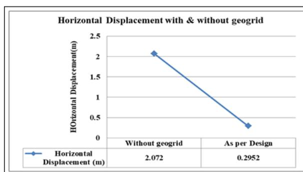
**Figure 4:** Variation in Horizontal Displacement of Embankment with and without Geogrid
