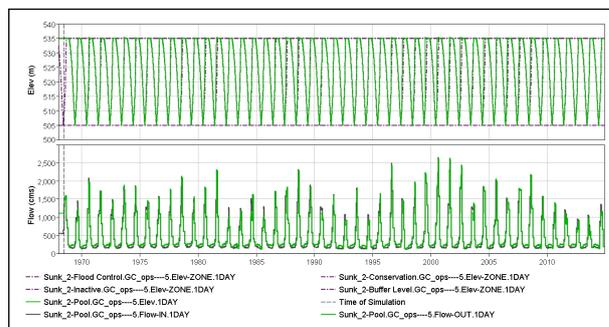
**Figure 6:** Reservoir elevation and inflow-outflow curves generated by reservoir Sunkoshi II operating in Alternative 5 policy of Scheme 2
