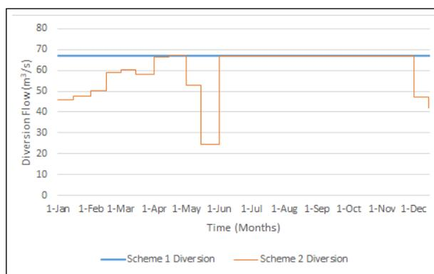
**Figure 7:** Sunkoshi Marin Diversion Multipurpose Project Release in two Schemes I and II
