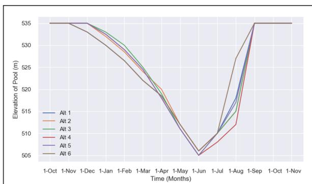
**Figure 3:** Alternative operation rule curves used in the Sunkoshi II
