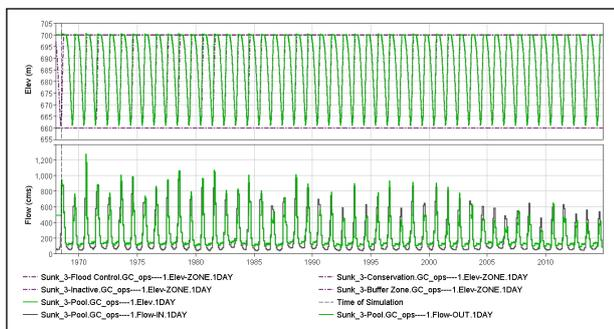
**Figure 4:** Reservoir Elevation and Inflow- Outflow curves generated by reservoir operation policy of Alternative 1 in Sunkoshi III of Scheme 1
