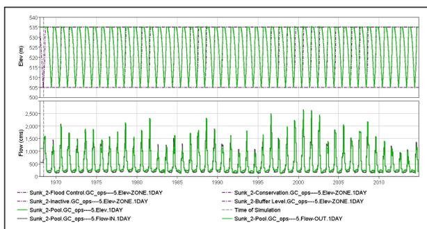
**Figure 5:** Reservoir Elevation and Inflow- Outflow curves generated by reservoir operation policy of Alternative 5 in Sunkoshi II of Scheme 1
