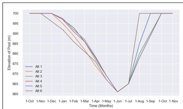
**Figure 2:** Alternative operation rule curves used in the Sunkoshi III
