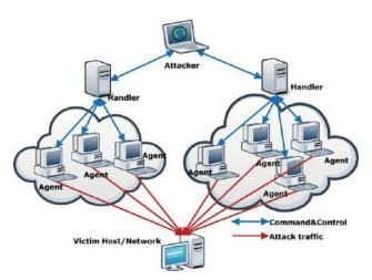
Figure 1: Flow Diagram of DDoS Attack
