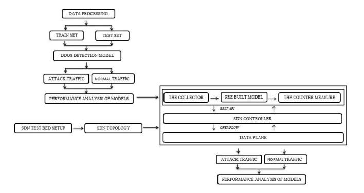
Figure 3: The System Block Diagram
