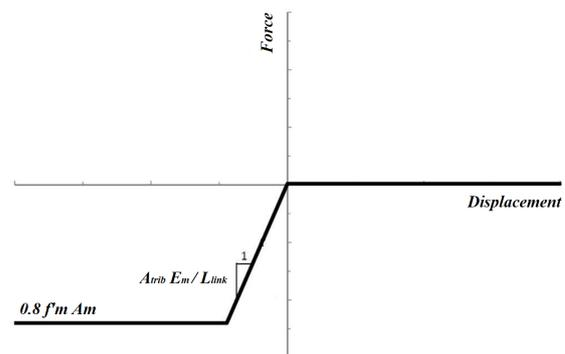
**Figure 1:** Nonlinear Link Definition for URM Wall, Axial Direction
