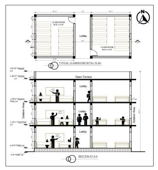
**Figure 10:** Typical Classrooms floor plan and Detail section of Gyanodaya Secondary School
