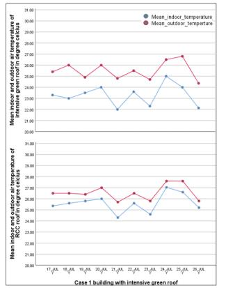
**Figure 9:** Comparison of mean indoor and mean outdoor air temperature of case 1 building.
