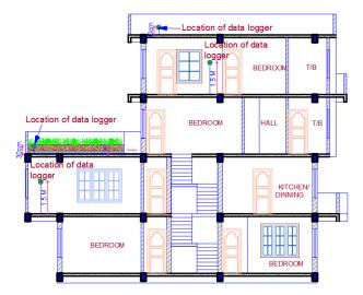
**Figure 2:** Building section of case 1 building with locations of data logger in indoor and outdoor of building for air temperature measurement.
