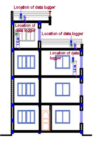
**Figure 6:** Building section of case 3 building with locations of data logger in indoor and outdoor of building for air temperature measurement.
