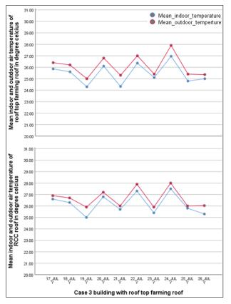
**Figure 11:** Comparison of mean indoor and mean outdoor air temperature of case 3 building.
