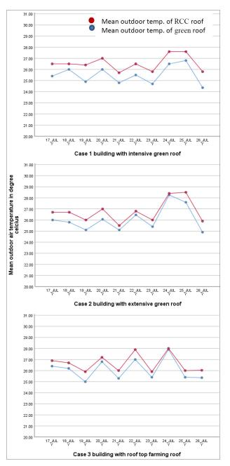
**Figure 8:** Comparison of mean outdoor air temperature of green roof with RCC roof.
