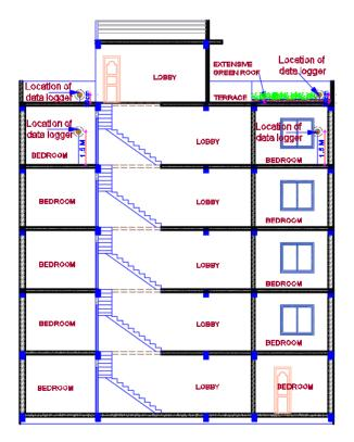
**Figure 4:** Building section of case 2 building with locations of data logger in indoor and outdoor of building for air temperature measurement.
